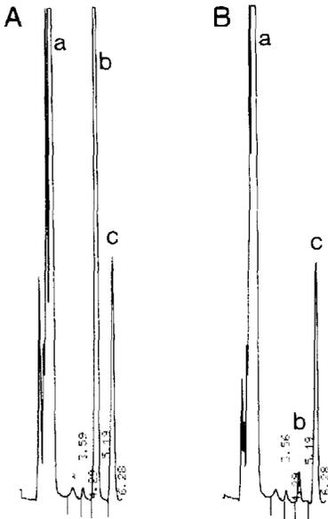
Fig. 2. HPLC of incubated (A) blank plasma and (B) plasma spiked with benazeprilat (600 pmol/ml). Peaks: a = hip-hist-leu; b = hippuric acid (RT = 5.19 min); c = mandelic acid (RT = 6.28 min).
