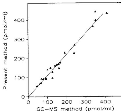
Fig. 5. Correlation of benazeprilat concentrations measured by the enzyme inhibition-HPLC method and by GC-MS [4] in plasma of volunteers administered benazepril·HCl.  $y = 1.16x - 1.90$ ;  $r = 0.998$ ;  $n = 9$ .
